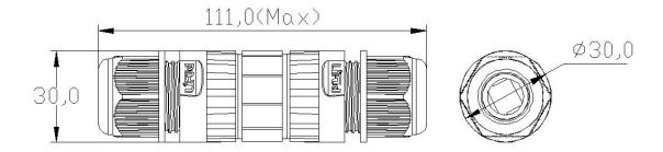
\* The wire outlets are compatible with two-core or three-core cables of 22# to 16# rubber or sheathed wires. (Expose 4mm to 6mm wire core. Peel 14mm to 16mm sheath. Use cables with the diameter of 5mm to 8mm.)
